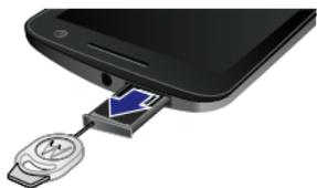
2. Put the nano SIM card in the tray with the gold contacts facing up. Turn the tray over to put in a microSD memory card.
